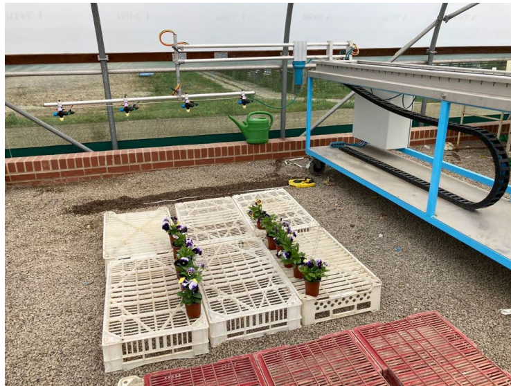
Figure 16 Plants arranged in two lines in the centre of the three nozzles in use by the precision track sprayer
